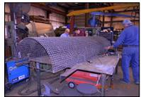
Scale Model of Breakwater Frame
