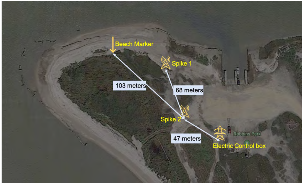
Figure 6 Preliminary lay out for Smith Point Station. Spike 2- proposed location for CODAR enclosure); Spike 1- proposed location for antenna; Electric Control box is location of pre-existing source of power.
