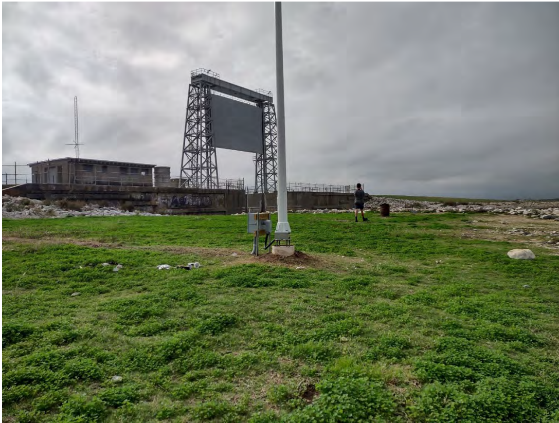
Figure 11 Installed SeaSonde antenna at Moses Lake Tide Gate. Electronics are housed in gate control build in background
