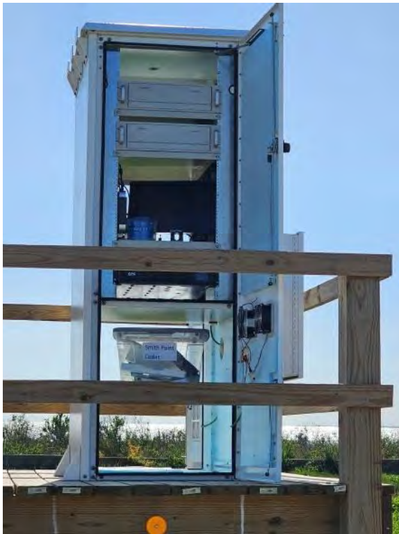
Figure 17 View of installed SeaSonde electronics inside climate-controlled enclosure
